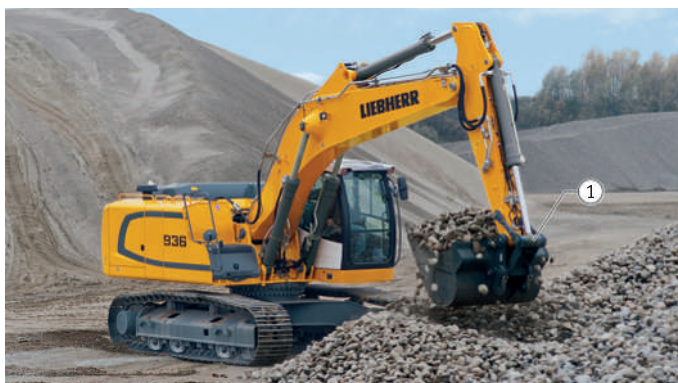
27 Application example with high wear load: Spherical plain bearing in excavator
